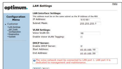
3. Optional: Enable the DHCP server. This will allow the SIP Trunk Adaptor to act as a DHCP server, which will provide IP addresses to the voice network, and create a dedicated voice LAN, as per diagram 2.
