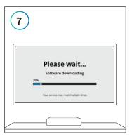
Release the power button when you see the "Software downloading" screen. Allow up to 10 minutes for your Mini to configure. It will turn on and off several times during the process.
