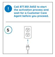
When you've reached an Agent, plug the Mini power cord into an electrical outlet.
